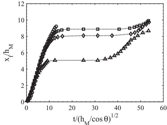
FIG. 6. Influence of the channel width on the normalized granular front position as a function of the normalized time. Experimental measurements refer to the case of waves over rigid, flat beds, when  $\xi_0 = 0.75$ , for  $W = 18$  (open triangles),  $W = 37$  (open diamonds),  $W = 62$  (open squares), and  $W = 123$  (open circles).
