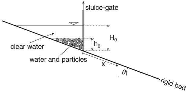
FIG. 1. Sketch of the experimental setup and the initial configuration.
