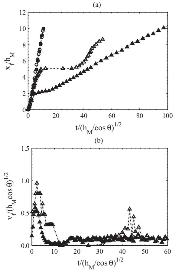
FIG. 4. Influence of the channel bed on (a) the normalized granular front position and (b) the normalized granular front velocity as functions of the normalized time. Experimental measurements refer to the case of waves in a channel of  $W = 18$ , for  $\xi_0 = 0.75$  and flat bed (open triangles),  $\xi_0 = 0.75$  and bumpy bed (filled triangles),  $\xi_0 = 1.25$  and flat bed (open circles), and  $\xi_0 = 1.25$  and bumpy bed (filled circles).
