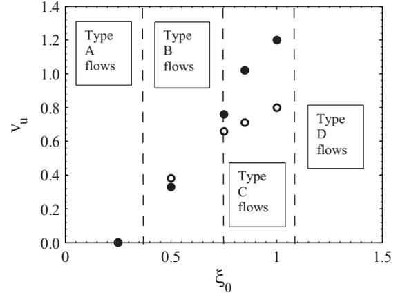
FIG. 7. Granular front velocity at the uniformly progressive state as a function of the initial degree of saturation for flows over bumpy beds, when  $W = 18$  (filled circles) and  $W = 123$  (open circles).
